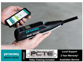
Conversion curves are provided for a wide range of concrete compressive strength, including low and high strength concrete fc <10 MPa (5MPa using Mushroom Head) and up to 100MPa.
