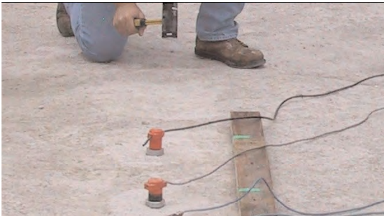
Typical SASW-G test setup for a close-spacing test using 4.5 Hz geophones on pavement
