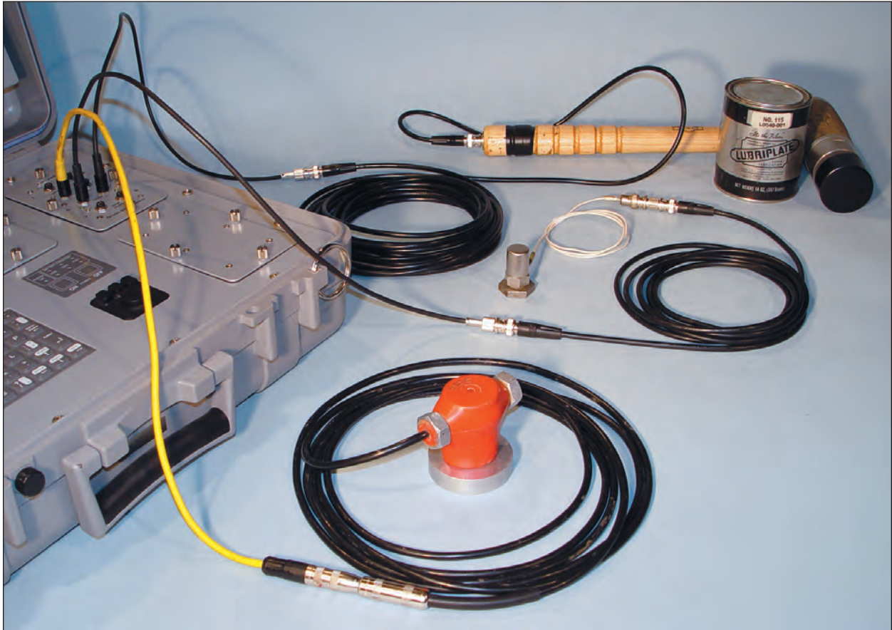
Complete SE/IR System with Accelerometer showing all components properly attached
