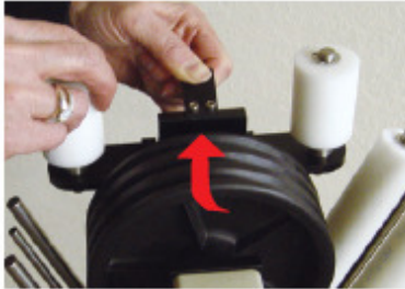
13a -Squeeze latch spring and rotate pinch roller assembly upward
