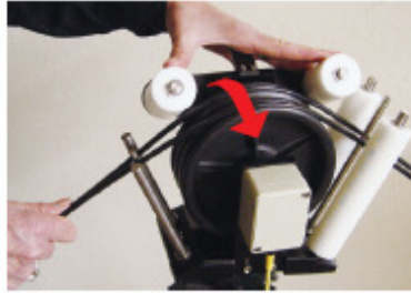
13b - Holding wires, rotate pinch roller assembly back to LOCK
