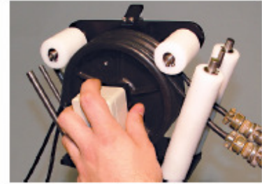
13c - Slack adjusted in cable, rollers in LOCK position.
