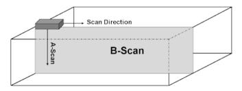
The spacing between A-Scans is entered in the "Settings" menu. Position the transducer at the starting position.
