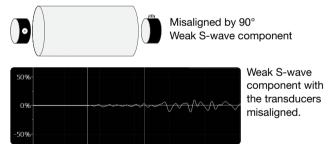
Rotate one transducer into and out of alignment and watch the S-wave component increase and decrease.
