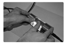
Couple the transducers to the Calibration Rod (F) using the ultrasound Couplant (E) and press firmly together.
