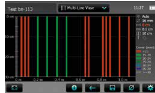
Figure 19: Multi-Line View with cover values displayed
