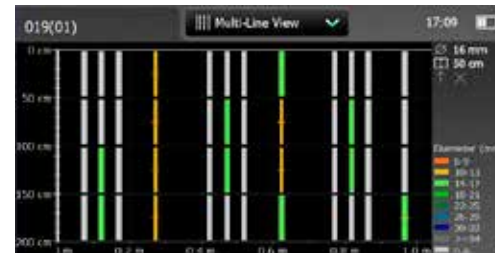
Figure 20: Multi-Line View with diameter values displayed (if measured)
