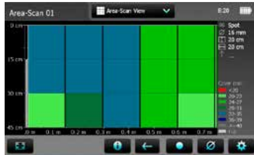
Figure 23: Area-Scan View (zoomed to show X- and Y-axis in the same scale)
