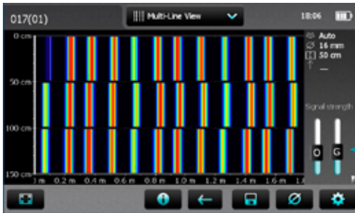
Figure 21: Multi-Line View with Signal Strength color spectrum
