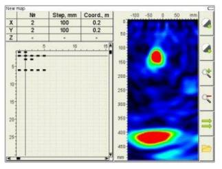
This mode is used to take multiple scans over a proscribed Grid. This data can be processed into 2D or 3D images with Ideal Viewer. Each scan is displayed as a 2D image similar to that produced by Investigation Mode.
