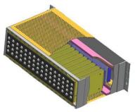
Each measuring unit consists of 4 lowfrequency broadband DPC transducers with the nominal operation frequency of 50 kHz, These produce shear waves using only a dry point contact. The transducers have wearresistant ceramic pins,
