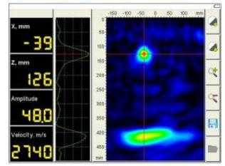
This mode is for quick data acquisition and spot checks, a single measurement is taken and can be recorded as an Image file. This mode is used to change settings to provide clear imaging of the internal structure of the concrete and to work quickly onsite.
