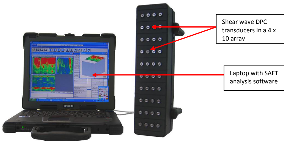
Figure 2- View of the Shear wave ultrasonic tomography MIRA System
