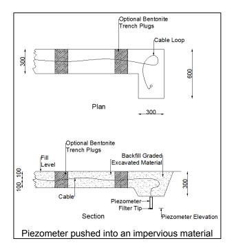
7. Having prepared the piezometer for installation and recorded its site Zero Reading (see Section 5.1), bring it to site for installation in a water filled
