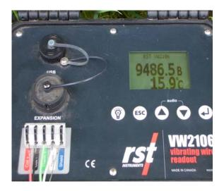
Record the values displayed on the readout ( and units ) against the piezometer serial numbers. If these 'out of the box' CHECK readings show significant differences ( +/- 40 digits ) to the zero pressure values on the calibration sheets, contact MGS Geosense for assistance. ( It should be noted that the 'CHECK Readings WILL be affected by the atmospheric pressure & altitude ).
