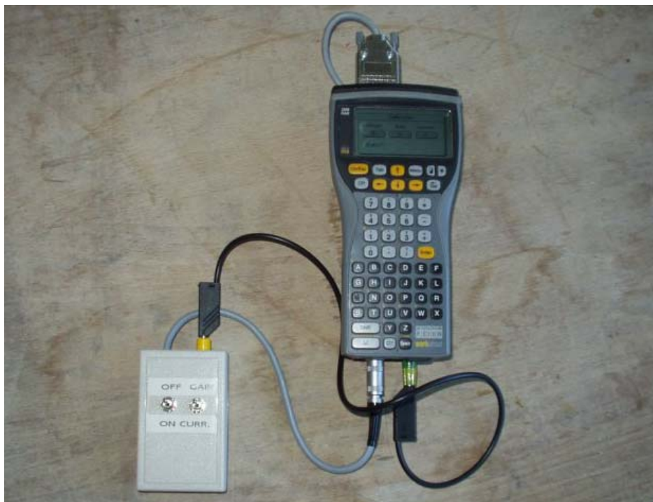
Fig 17. PSION and calibration box connected ready for calibration
