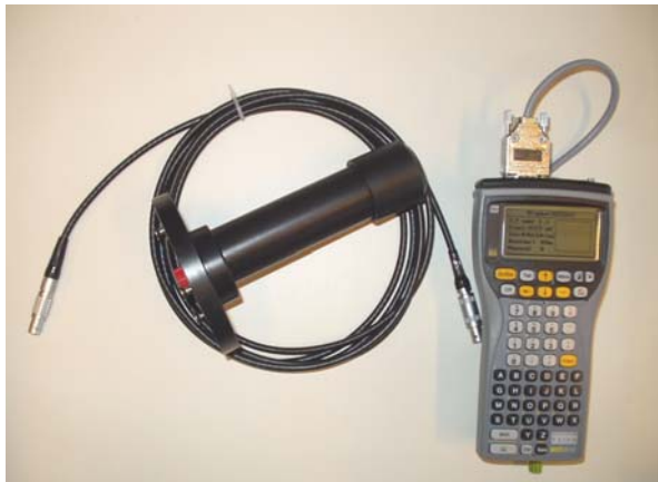
Fig. 35. Connection cable, electrode and GalvaPulse computer
