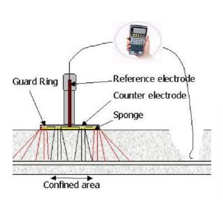
Figure 1. Sketch of GalvaPulse™ electrode
