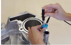
Figure 4: Leeb Testing Procedure
