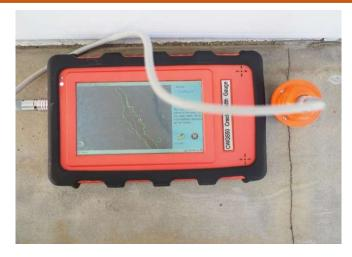
**Crack Width Measuring Camera**
