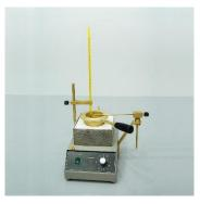
and a thermometer. To conform to the CE European Directive, the unit comes complete with a double line-fuse, Hot plate control apparatus and a thermometer -6 C to +400 C.
