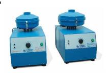
cylindrical aluminium box. An electric motor fitted with an AC drive (inverter) drives the bowl. The motor has the double function of speed control up to 3600 rpm regardless of the frequency (50 or 60 Hz) and electrical breaking. The centrifuge can be set for the automatic speed ramp up to 3600 rpm and will stop in 10-15 seconds.
