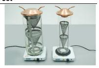
The extractor uses the difference between the weight of extracted aggregates, moisture content and ash from an aliquot part of the extract to determine the bitumen content.
