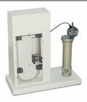
the measuring cell is 41 mm in diameter.
