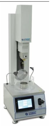
situated on the front panel, the position of the needle can be adjusted. An ultra-bright LED lamp and a magnifying glass come supplied with the apparatus. The plunger is then automatically released onto the sample, and once the test is finished, it is raised automatically. The test result is displayed on the digital display. The user can easily remove the plunger, if the weight needs to be calibrated.
